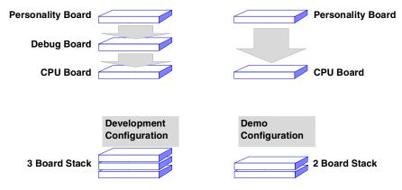
Figure 3.1 3-Stack Platform Configurations
